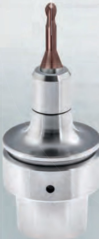
Short shank tool with adapted shank length 21 – 26 mm (for Ø 6.0 mm)
